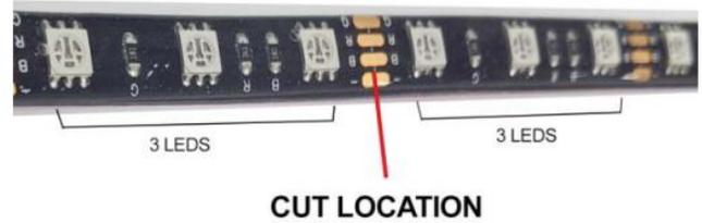
The LED strip can be cut one time on the copper solder pad where indicated; between the cluster of 3 LEDs. Important to cut in the center of the copper pads. Once cut, the end must be sealed using silicon, liquid electrical tape or even heat shrink to stop water intrusion from damaging the strip.
