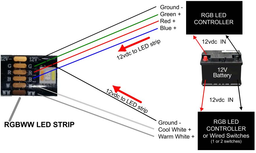
The RGBWW LED Strip has 5 diodes: Red, Green, Blue, Warm White, Cool White. You can power those 5 diodes using a single RGBWW LED Controller or you can power them using a combination of 1) RGB Controller + Hard Wire Switch(es) or 2) RGB Controller + RGB Controller. In all cases, the ground has to be supplied to each controlling device as shown in the above diagram.
