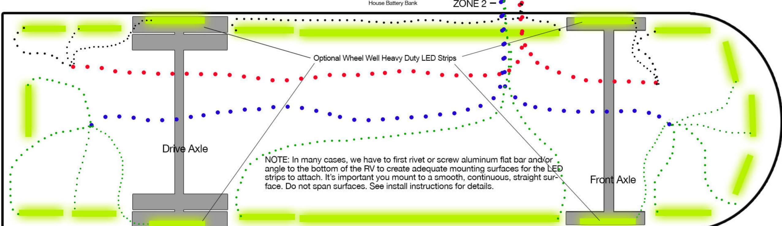
All power leads must run back to the Boogey Lights LED controller mounted at or near the 12vdc power source. We always recommend using the house batteries as the power source. IMPORTANT! LED strips can not "daisy chain" from one strip to the next. NOTE: LED Strips can be cut every third LED if you need shorter lengths.
