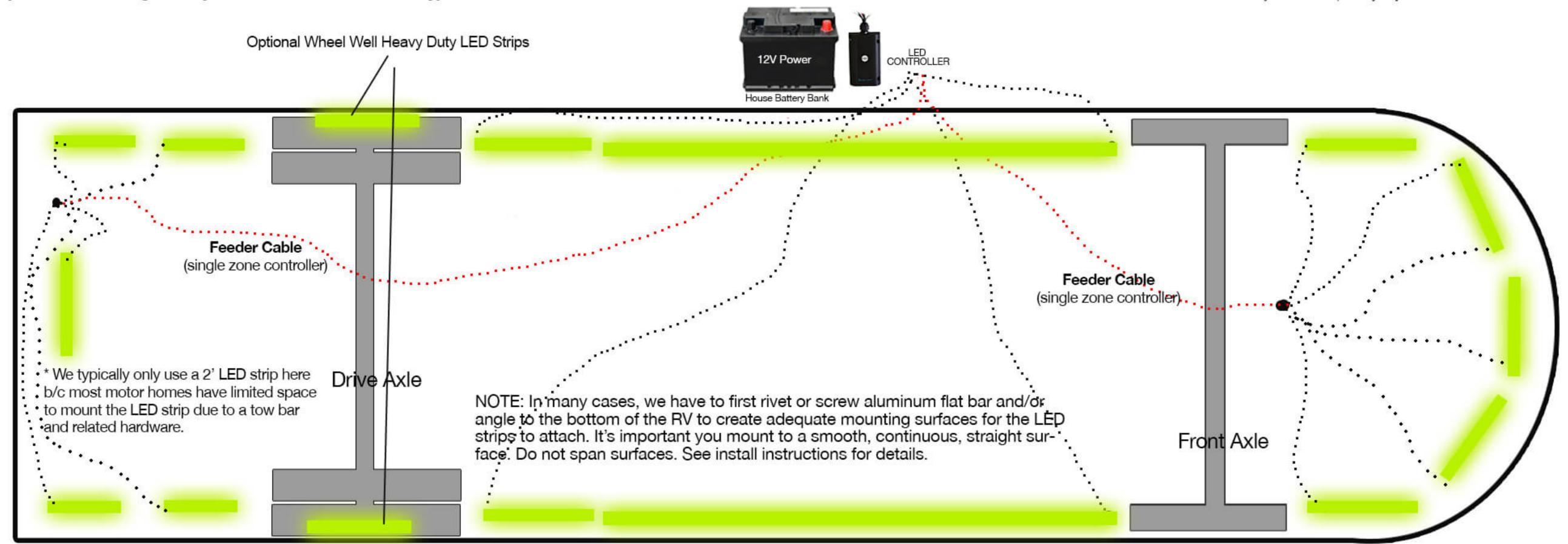
All power leads must run back to the Boogey Lights LED controller mounted at or near the 12vdc power source. We always recommend using the house batteries as the power source. IMPORTANT! LED strips can not "daisy chain" from one strip to the next. NOTE: LED Strips can be cut every third LED if you need shorter lengths.
