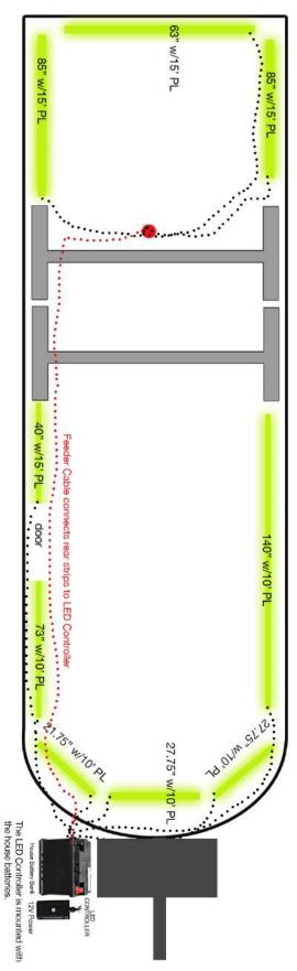
All power leads must run back to the Boogey Lights LED controller mounted at or near the 12vdc power source. We always recommend using the house batteries as the power source. IMPORTANT! LED strips can not "daisy chain" from one strip to the next. NOTE: LED Strips can be cut every third LED if you need shorter lengths.
