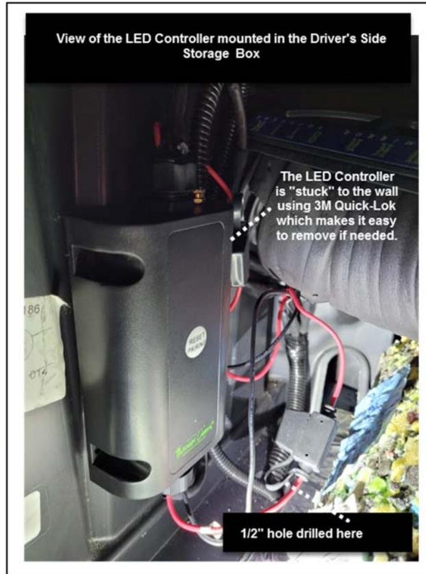
NOTE: The photos here are of our HEAVY DUTY LED CONTROLLER which is used for large LED installations which typically include Under-Glow and/or Under-Cab lighting systems. For the Western Star Grill and Air Vent kit, you won't have an LED controller this large.
