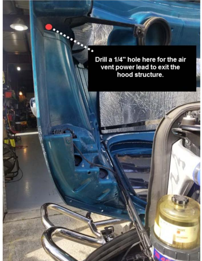
A 1/4" hole is all that's needed. We put down some Gorilla Tape first before drilling into the fiberglass. Helps reduce cracking/splintering.
