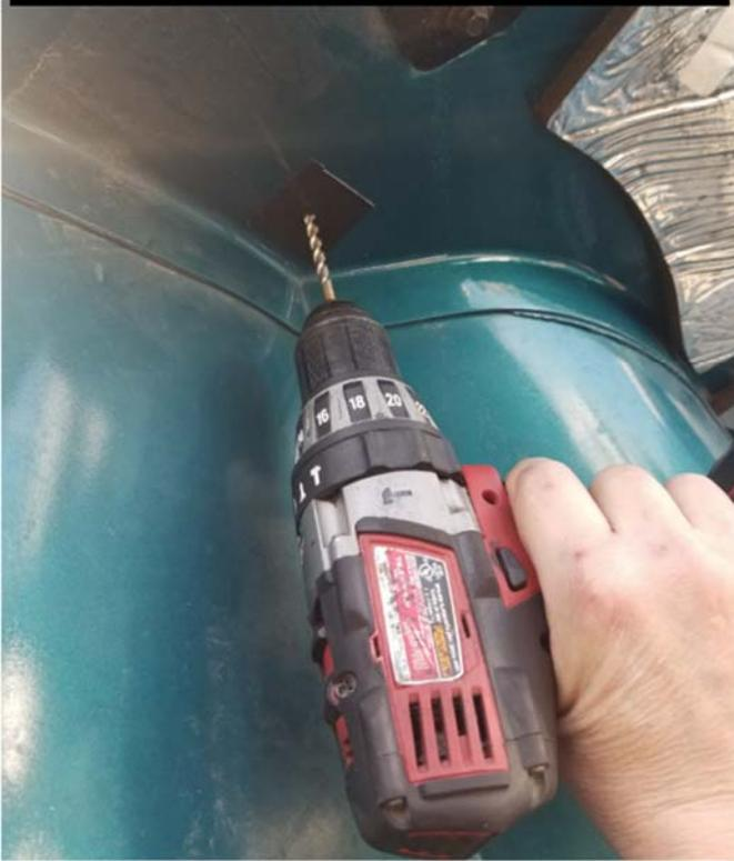
Close up view of the hole we drilled under the passenger's side air vent where the power lead exits the hood structure. We use Butyl tape to seal the hole.
