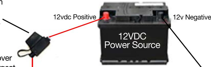
Instead of running the ground wires to the negative terminal on the battery, it's usually easier to connect the negative side of the LED strips to the vehicle ground. Just make sure there's a good ground by making sure you're connecting the ground wire to bare metal of the vehicle chassis (eg. no paint or rust.)
