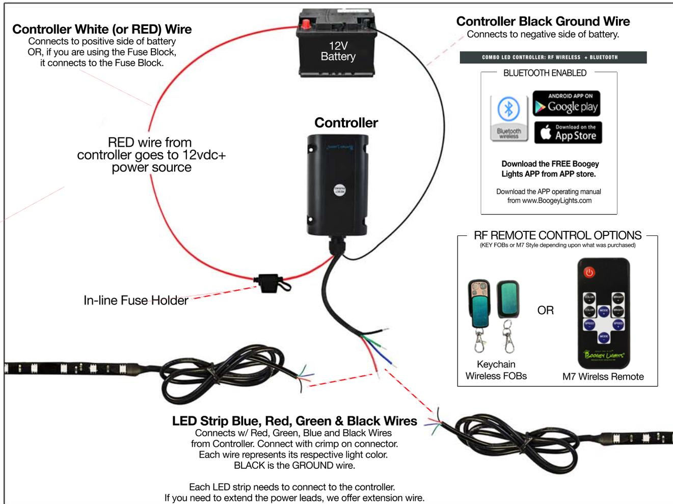
NOTE: If the distance from the LED Controller to the battery is more than 18", we strongly recommend adding another INLINE FUSE on the positive side of the circuit at the point at which the 12vdc+ connects to the battery.
