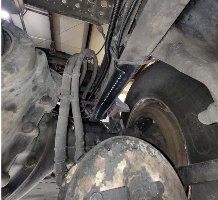
View of LED Segment 'I' mounted to the frame rail.
