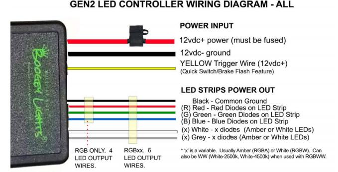
Important to cap (seal) the yellow trigger wire if not using the brake flash or quick switch feature.
