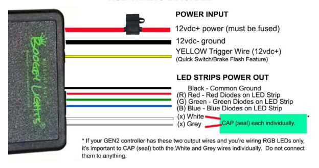
NOTE: If you have the PLUS version of our GEN2 LED controller, it is an RGB only controller and as such you won't have the white or grey output wires shown in the above diagram.
