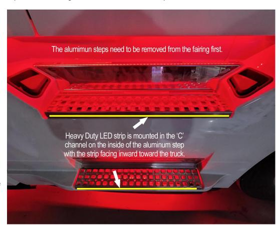
We recommend leaving an extra 2' or 3' of power lead slack on the back side of the fairing to allow for movement of the fairing when it is being removed from the truck for service.
