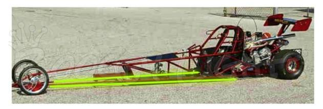
This frame structure can use one single LED strip on each side.
