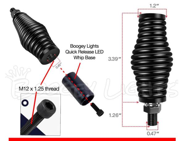
The base of the BOOGEY LIGHTS LED WHIP bolts into the top of the spring using the supplied M12 x 1.25 x 30mm allen head bolt with flat washer and lock washer. The LED whip base comes stock with a 10mm wide mounting hole. To use this heavy duty spring with the LED Whip you'll need to drill out that hole to fit the larger diameter 12mm allen head bolt. The base is made of aluminum so it's easy to do.
