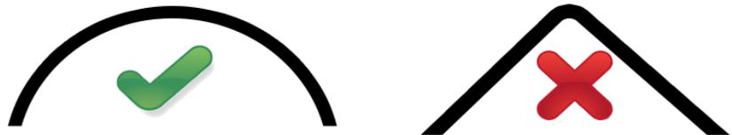
Do NOT bend the LED strip on a horizontal plane.
